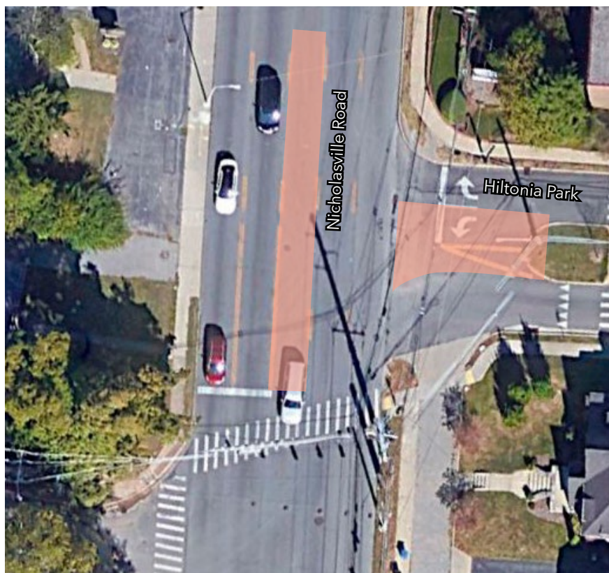
Figure 5.64 Median and right-in/right-out with bicycle through movement only, shown in pink
