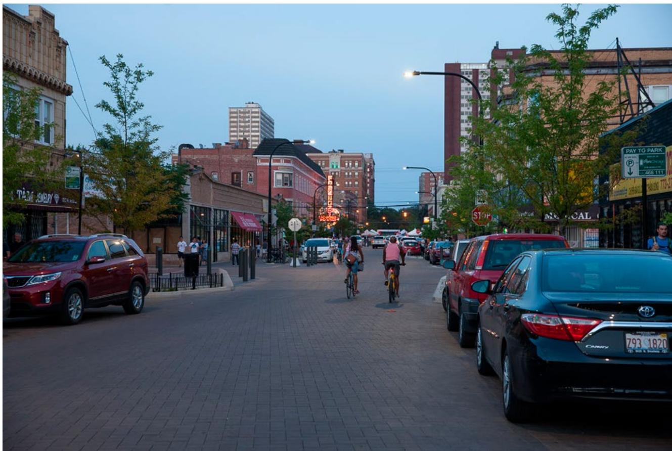
Figure 5.39 Two-way shared street example on Argyle Street in Chicago, IL. (Source: Site Design Group, Ltd.)
