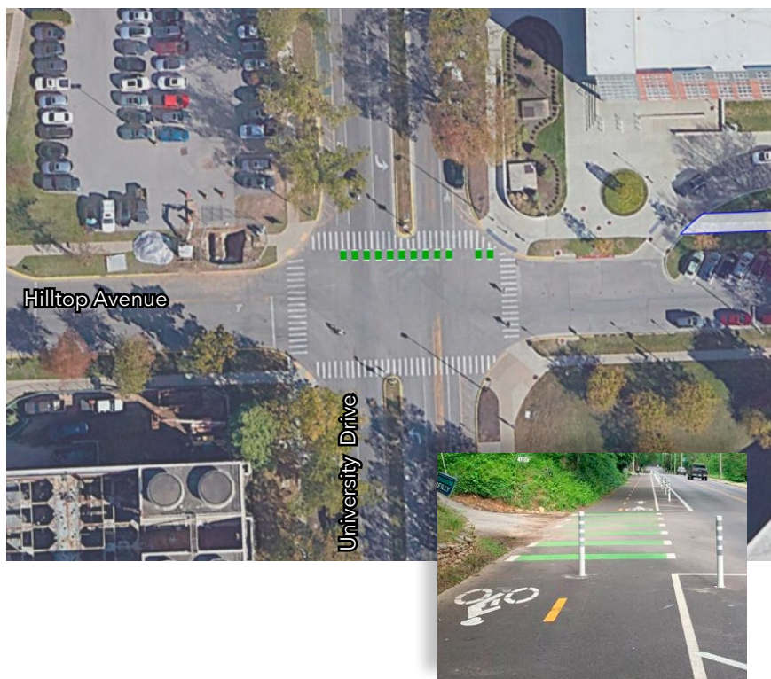
Figure 5.29 Protected intersection for right turning bicyclists at University Drive and Hilltop Avenue, featuring buffers like those shown in the inset.
